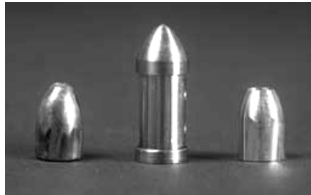
Figure 1: A master bullet from ATF National Laboratory Center (left), a NIST prototype standard bullet (center), and a NIST RM 8240 standard bullet (right).
