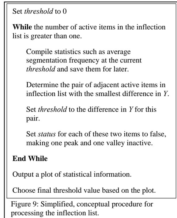
Figure 9: Simplified, conceptual procedure for processing the inflection list.
