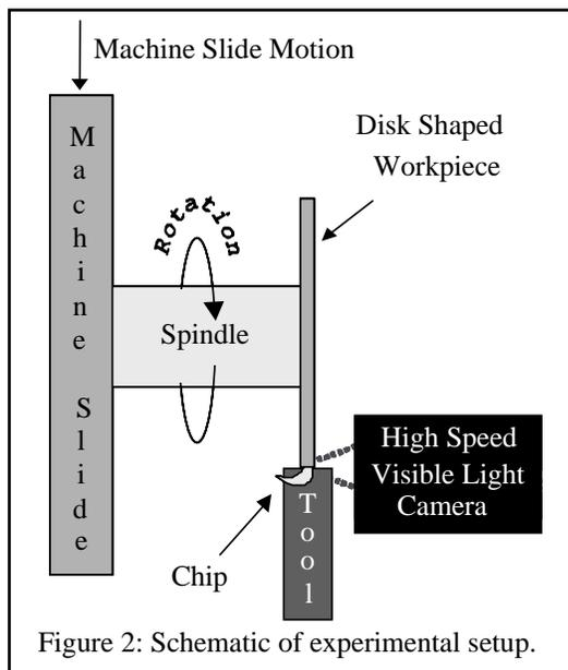
Figure 2: Schematic of experimental setup.
