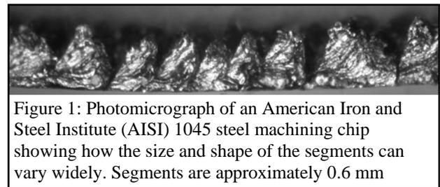
Figure 1: Photomicrograph of an American Iron and Steel Institute (AISI) 1045 steel machining chip showing how the size and shape of the segments can vary widely. Segments are approximately 0.6 mm
